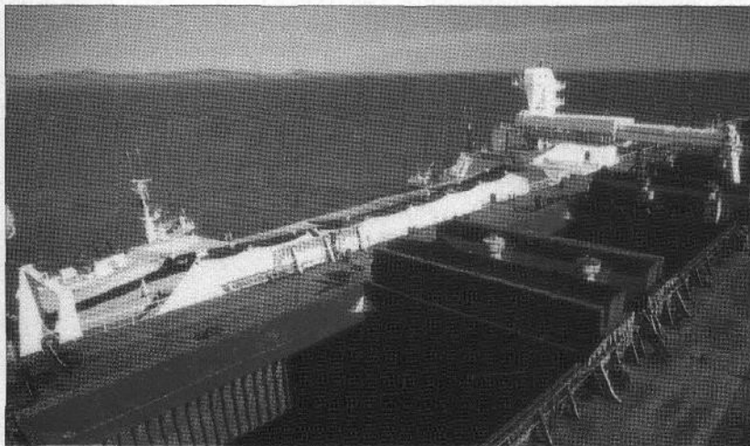
Lightering barge (background) loading ore onto a ship.
